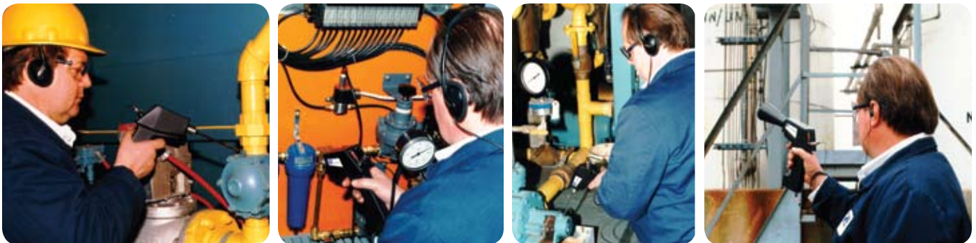
Left to right: Valve leakage, pressure / vacuum leaks, mechanical inspection and tank leakage.
